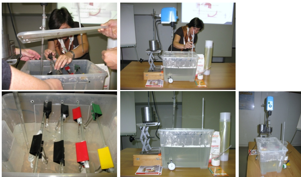
Picture 22: Prototype for whey layer removal by washing with enzymatic detergents
