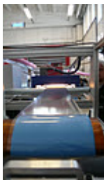
Picture 15: prototype coating and winding section
