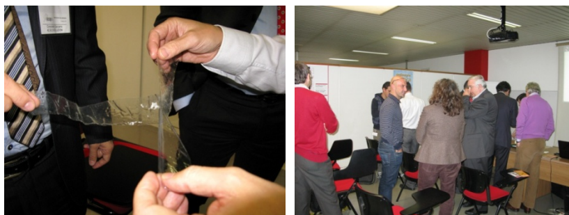
Picture 26: Film separated in the two layers of PET and PE.
