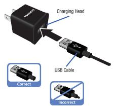
Note: Verify that the battery is installed prior to connecting the wall charger. If both the wall charger is connected and the battery is not installed, the handset will power cycle continuously and prevent proper operation. Failure to unplug the wall charger before you remove the battery, can cause the phone to become damaged.
