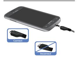
Note: This illustration displays both the correct and incorrect orientation for connecting the charger. If the charger is incorrectly connected, damage to the accessory port will occur therefore voiding the phone's warranty.
