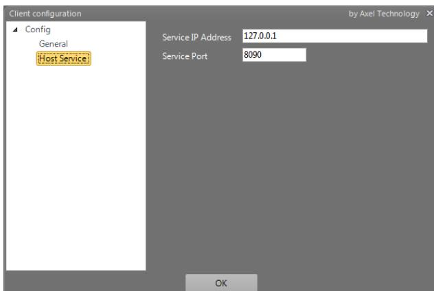
Set the IP address of the pc where XMUSIC service is installed and the port used by the service.
