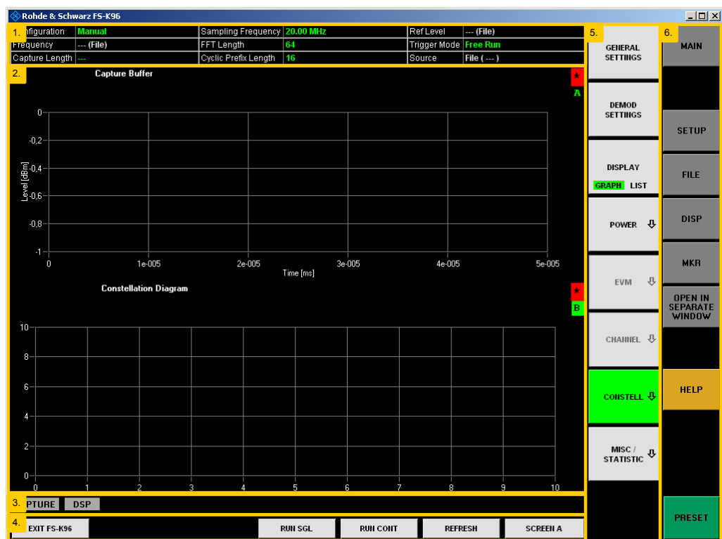
Fig. 1-1: Six Main Elements of the R&S FS-K96 Software
