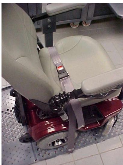
Examples of a Power Chair (left) and a Scooter (right) strapped to the platform
