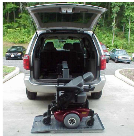
Power Chair on platform; seat back folded down to fit into vehicle
