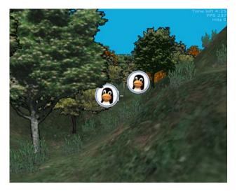
Fig. 3 The display of the FPS input device testing system used by Isokoski and Martin. Notice the two crosshairs. The big white one (on the left edge of the leftmost penguin tablet) was the standard FPS crosshair that stays in the middle of the screen. The small red crosshair (on the neck of the penguin tablet on the right) followed the gaze
