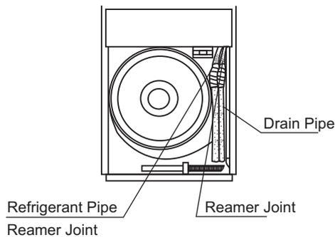
Pipe/wire-hole positions on both sides
