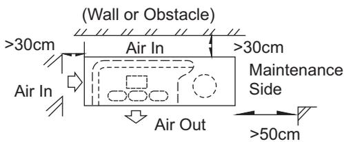
**When the air-out surface is facing a wall**
