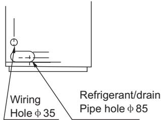
Pipe/wire-hole position on the bottom
