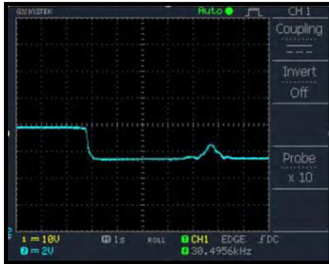
Figure 15: Impulse on Crack (Filter Output)
