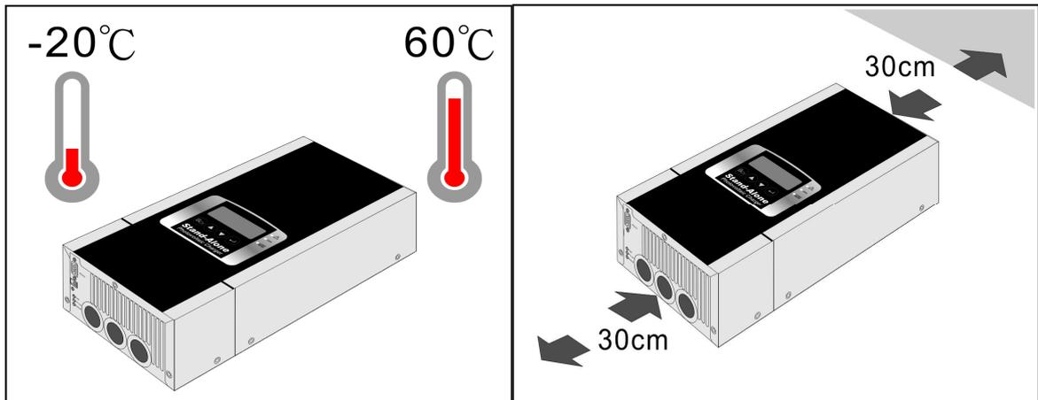
**Figure 2: Installation Environment**
