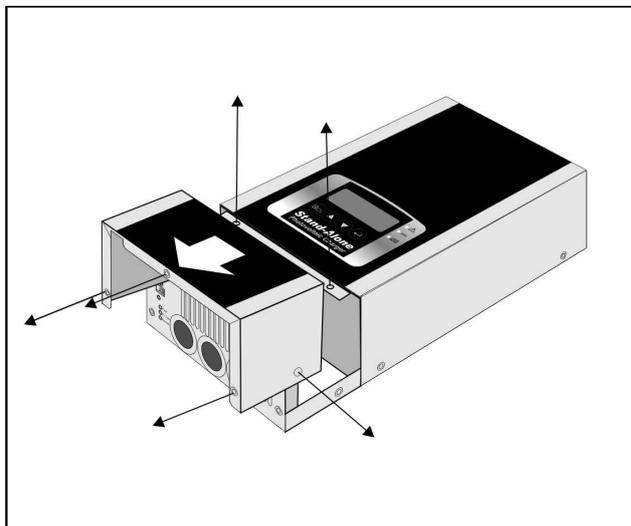
Figure 4: Remove Wiring Compartment Cover
