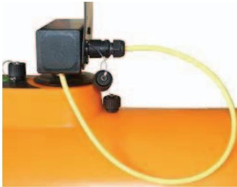
*Figure 19. Attaching the loop back cable.*
