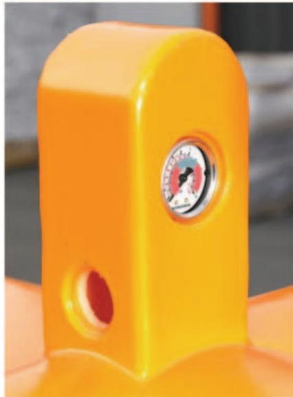
*Figure 4. Pressure gauge (on the Control Bridge).*
