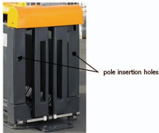
*Figure 5. Holes for insertion of transport poles.*
