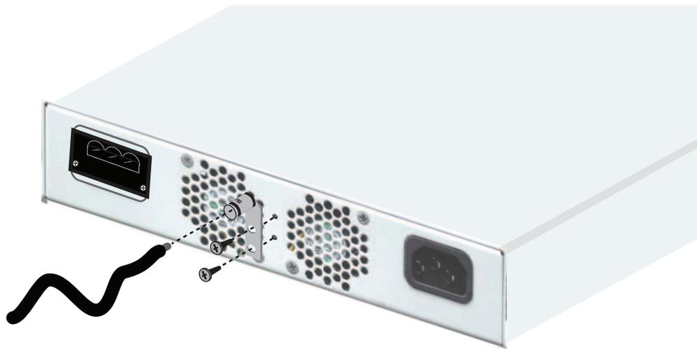
**Figure 3-12 Install Grounding Lug**
