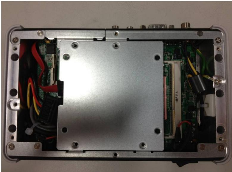
**Step 4** Loosen screws of HDD bracket
