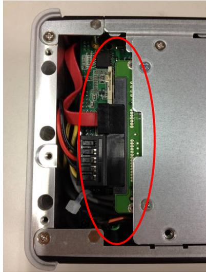
**Step 8** Close the HDD bracket to the chassis, and fasten all of screws.
