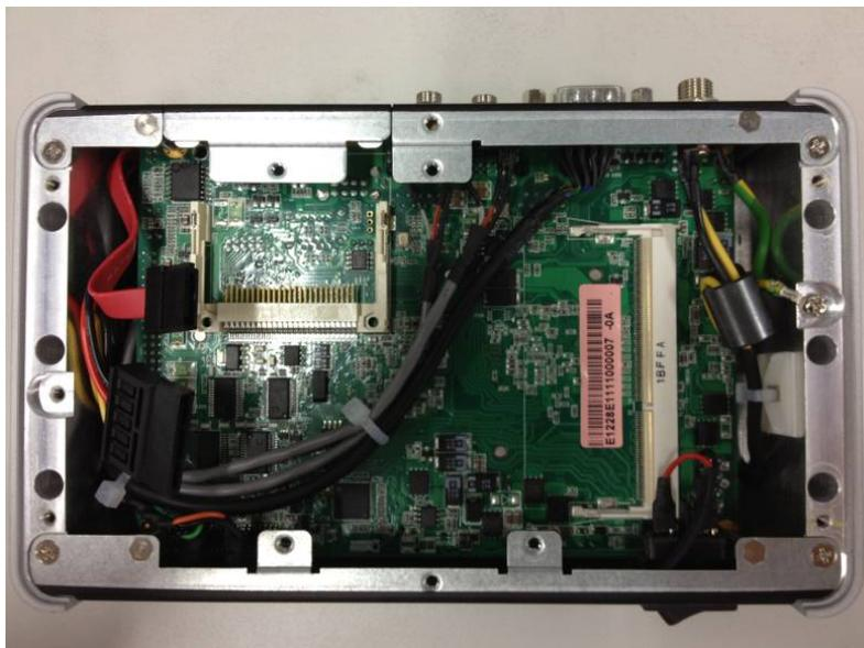
**Step 6** Locate the memory module, insert the gold colored Contact into the socket.
