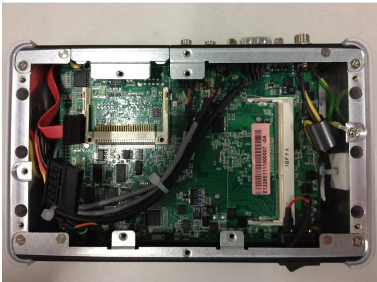
**Step 6** Assembly the HDD bracket together with the SATA HDD
