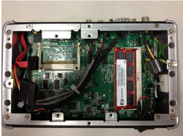
**Step 7** Push the module down, until it is firmly seated by locking two latches on the sides.
