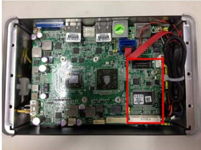
**Step 5** Slide Mini cards into Mini Card slot with caution and Fasten screw of Express Mini Card.
