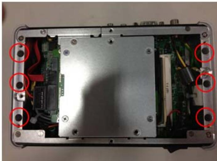
**Step 4** Remove the top heat sink to locate the PCI-Express Mini Card slot.
