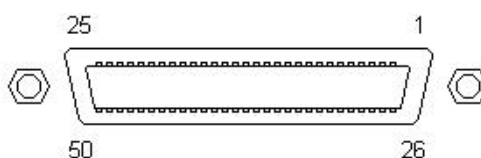
Figure 2-3 - RJ-21 Female-Type Telcom Connector
