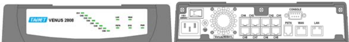
Figure 1-10 - The Front and Rear view of VENUS 2808S
