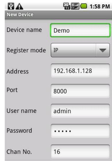
The screenshot shows the 'New Device' configuration screen with the following values: Device name (Demo), Register mode (IP), Address (192.168.1.128), Port (8000), User name (admin), Password (masked with dots), and Chan No. (16).
