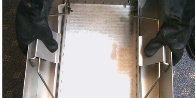
Locking latches on hold-down ring.
