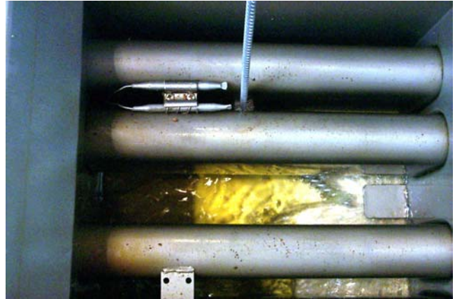
Use the L-shaped brush to loosen debris as oil drains from the frypot.
