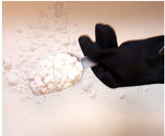
Use a measuring cup or scoop to evenly distribute filter powder over the filter sheet.
