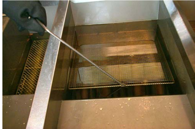
Removing support grid from frypot prior to draining.
