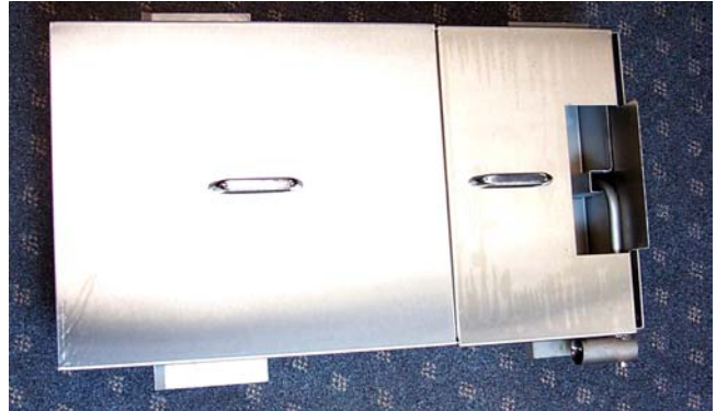
Pan covers properly placed.
