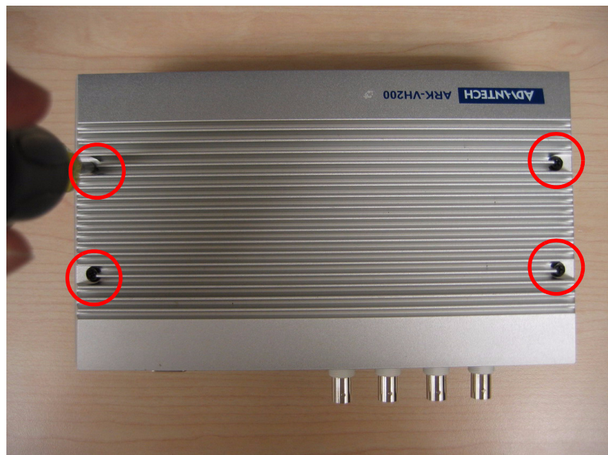
Figure 2.26 Unscrew the top case screws
