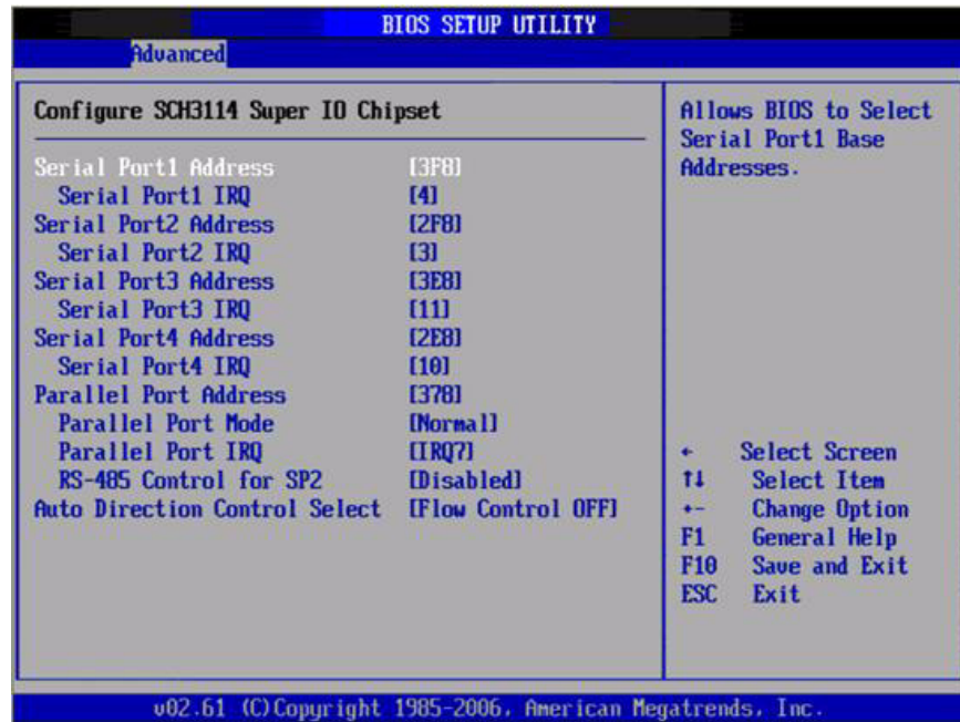
Figure 3.6 Super I/O Configuration
