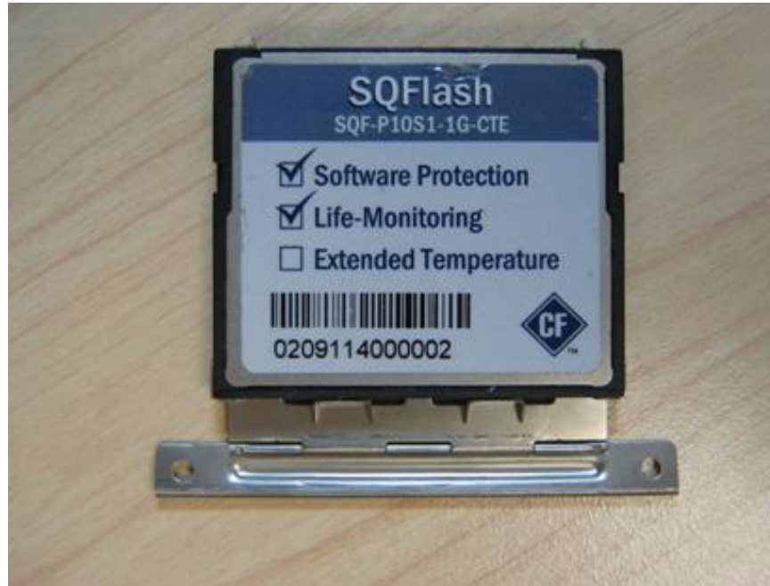
Figure 2.25 Put CF onto the CF tray
