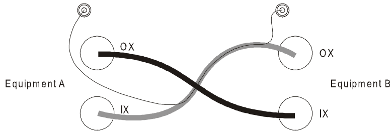
Figure 8 - Connecting the Messenger Wire
