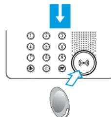
In case of a technical alarm (its symbol appears), you can find out which device has produced the alarm and reset it as well.
