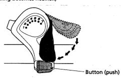
Push the button to shift to each of the gears.
