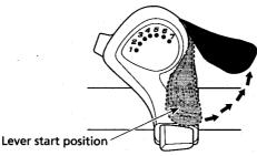
Push the lever to shift to each of the gears.
