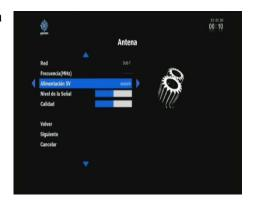
If you see a message like this on the screen it means there is a short circuit. Disconnect the receiver and check installation.
