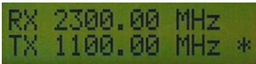
Figure 15: Transmitter Mode.
