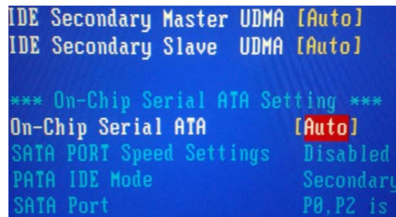
Figure 3-6 Select 'Auto' for On-Chip Serial ATA
