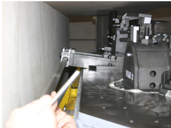
Figure 40 – Safety Devices 0501 and 0515, position adjusting with the Shaft Extension
