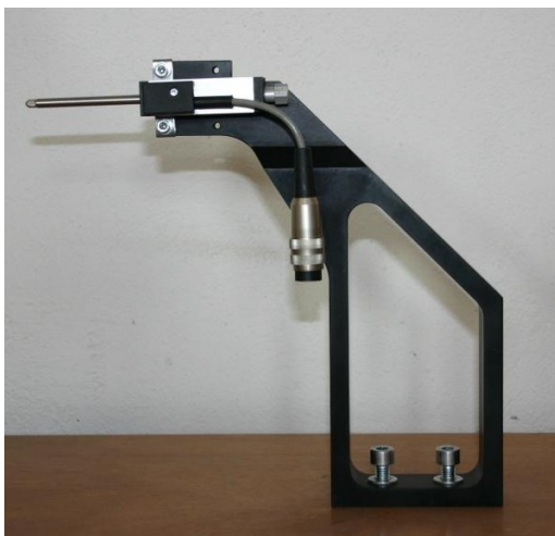
Figure 43 – Radial Absolute Transducer: apart and integrated
