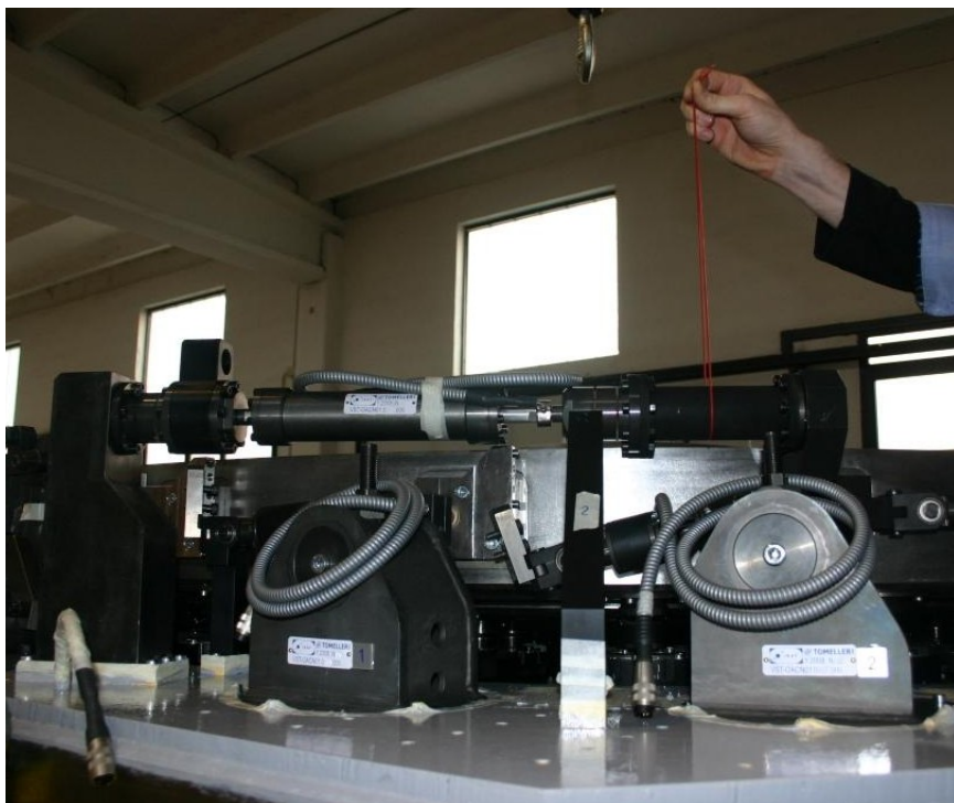
Figure 61 – Lateral Fixed Point supported by means of a string
