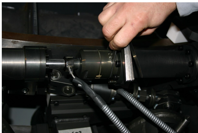
Figure 29 – Lateral Fixed Points, verifying the gap of the four flexible plates
