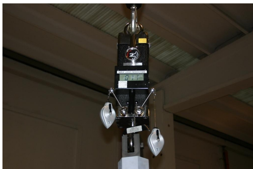
Figure 5 – hydra set for load monitoring when lifting the mirror
