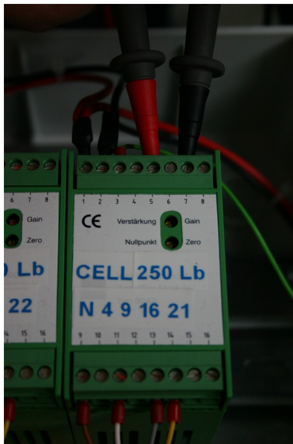
Figure 50 – Lateral Supports, Load Cell Amplifier: connections
