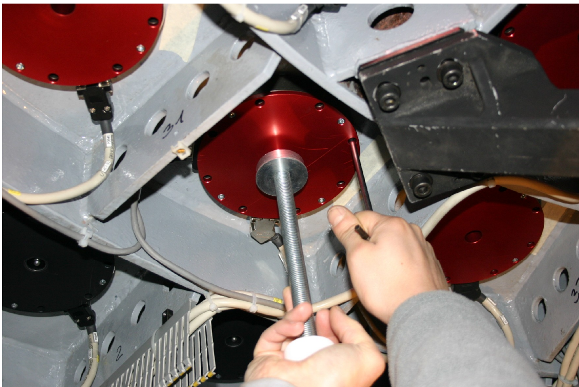
Figure 24 – Axial Force Actuator held with the Support Rod
