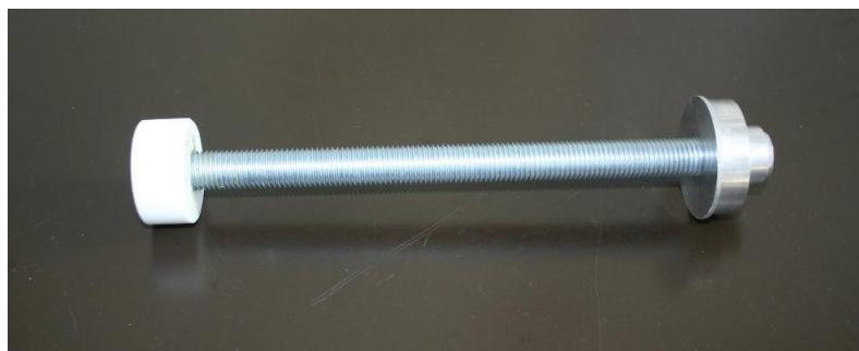
Figure 16 – Support Rod for the axial force actuators and axial fixed points
