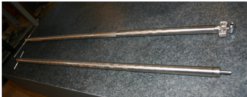
Figure 17 – Shaft Extension (bottom) and Key Extension (top) for safety devices 0501 and 0515
