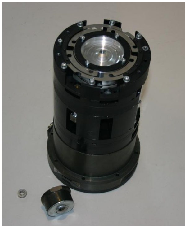
Figure 59 – Axial Force Actuator, top side view with sphere and spacer removed
