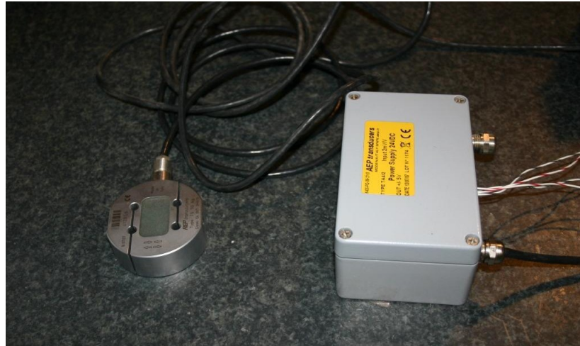
Figure 13 –high accuracy, 50kg full scale Load Cell
