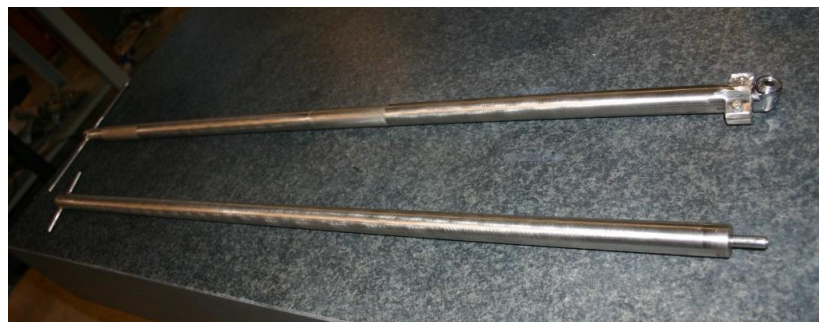
Figure 57 – Shaft Extension (bottom) and Key Extension (top) for safety devices 0501 and 0515
