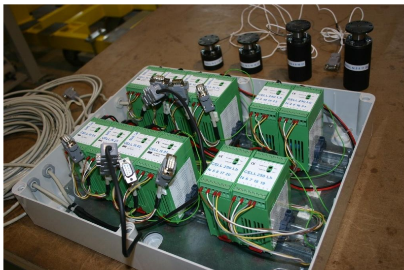
Figure 7 – Calibration Box with load cells and cables
