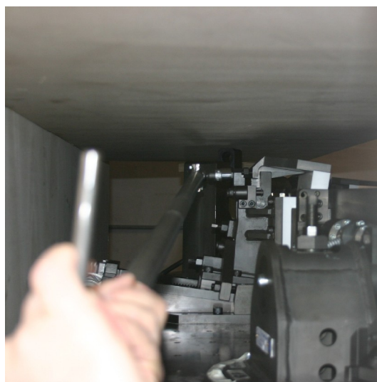
Figure 41 – Safety Devices 0501 and 0515, top arm adjusting with the Key Extension
