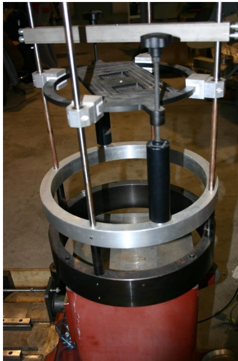
Figure 10 –Test Bench for the static tests (T1 and T3) of the axial force actuators
