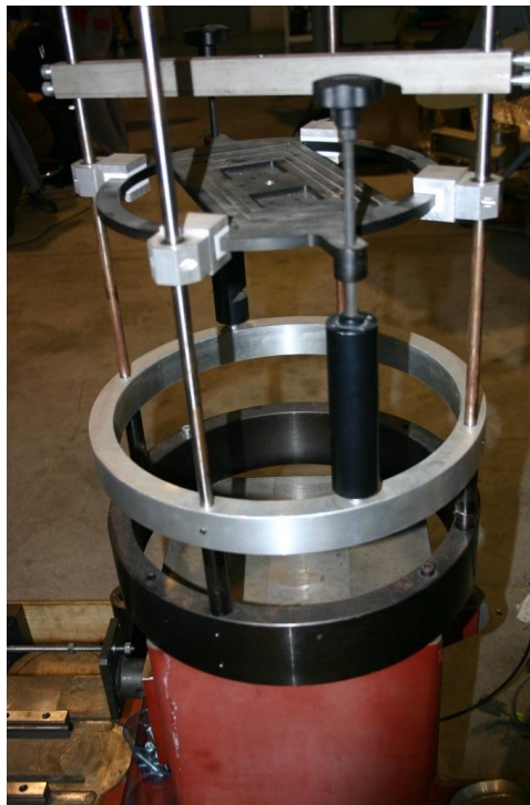
Figure 66 –Test Bench, to be used for the Pad of the Safety Devices as well
