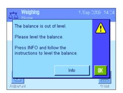
When the level sensor detects that the level is incorrect, the warning text at left will appear and a warning beep will sound. A status icon will also appear in the upper right-hand corner of the display (below the time).
