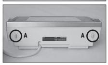
Now close the housing by pressing the two buttons (A) for adjusting the terminal until the housing base engages in the top housing.
