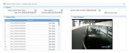
Select the corresponding control panel, door or network video recorder, input the start and end time, click [Search the Video] button. If the record matches the condition, the record number and name will display on the list, and the play and stop operation is permitted.
