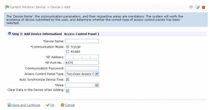
**IP** address: Please enter the IP address of the access control panel;
