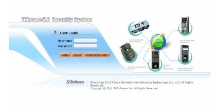
Before accessing the system, for system security, it is required to verify identity. We will provide a super user (having all operation levels) for the beginner of this system. Enter user name and password, and click [login], or click [Fingerprint Login], and then press the administrator fingerprint on the fingerprint sensor (need to install the fingerprint sensor driver first), to enter the system.
