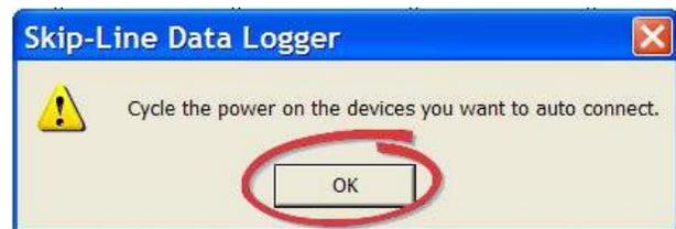
**4. Cycle the power on any wireless sensor modules on the truck you wish to associate with the logger system.**
