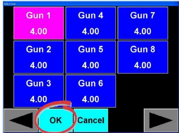
**3. Tap on the width that the gun is physically configured to, and tap "OK".**
