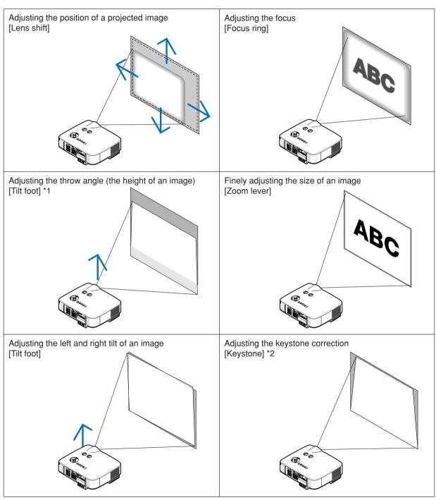
NOTE\*1: Adjust the throw angle (the height of an image) when the image position is higher than the lens shift adjustable range.
