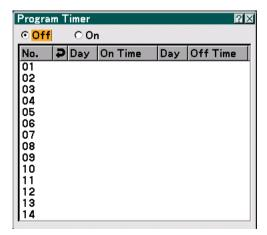
This option turns on or off the projector automatically at a specified time. Up to 14 different timer settings can be programmed.
