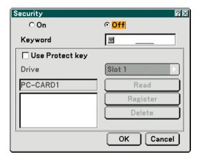
6. Press the SELECT ▼ button once to highlight the Keyword entry box and press the ENTER button. The Software keyboard will be displayed.
