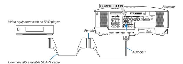
Before connections: An exclusive SCART adapter (ADP-SC1) and a commercially available SCART cable are required for this connection.
