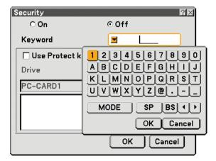
7. Enter an alphanumeric keyword using the Software keyboard For example, to enter "1234", follow the steps 7-1 to 7-4 below.
