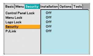
5. Press the ENTER button to display the Security screen.
