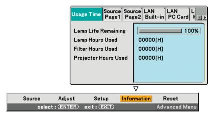
Displays the lamp and the projector usage hours, the status of the current signal and settings and LAN settings. This dialog box has seven pages.
