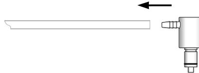
**Figure 10. Barbed Fitting on Tubing**
