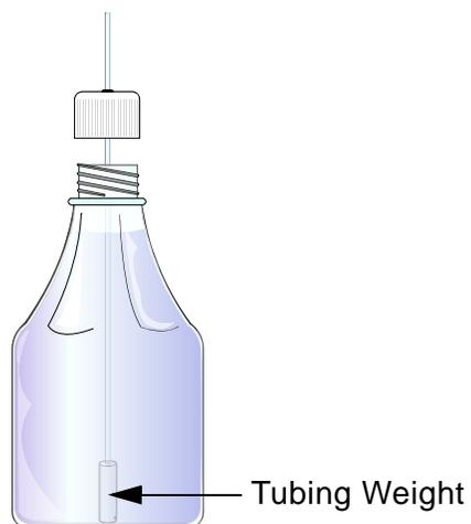
**Figure 4. Tubing Weight in Reservoir**
