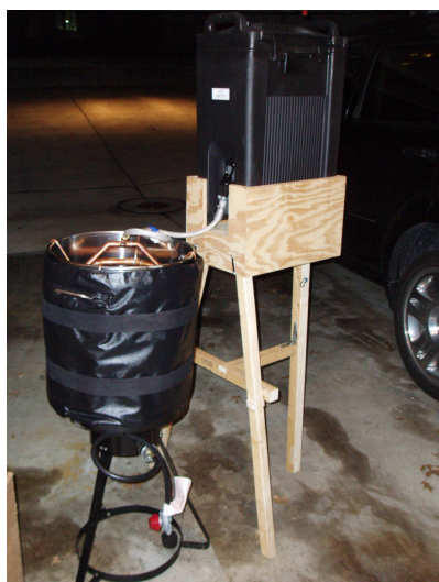
Fig. 5 Hot Liquor Tank on stand shown with insulated brewpot and brewpot stand
