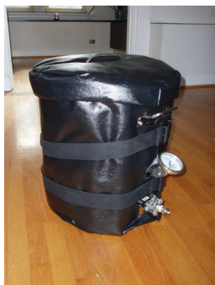
Fig. 7 Insulating jacket installed on brewpot and lid
