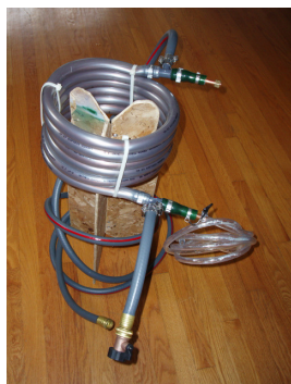
Fig. 12 - Silver snake, cooling water hose with shut off valve, wort hose and clamp and stand.
