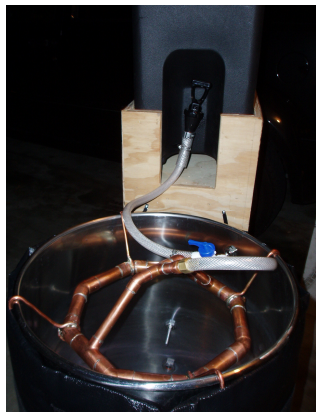
Fig. 6 Sparge ring shown in top of Brewpot, connected to sparge water tank
