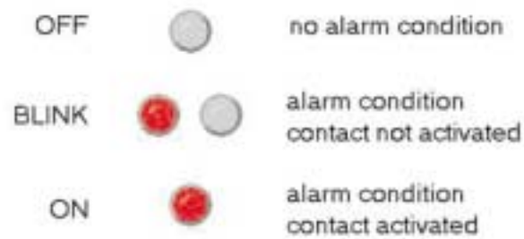
Figure 25 Alarm status indication
