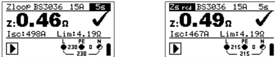
Figure 5.30: Examples of loop impedance measurement result
