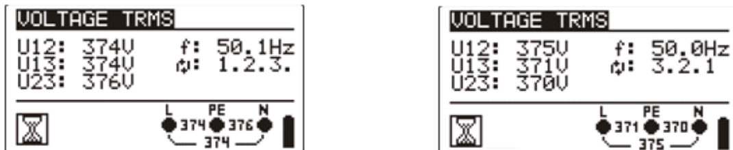
Figure 5.7: Examples of voltage measurement in three-phase system
