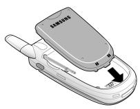
▶ To remove, make sure the power is off. Press the battery release latch up and remove the battery from the phone at a 45-degree angle.
