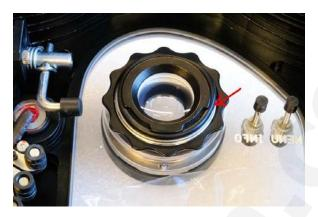
2. **Remove the viewfinder itself**: After taking off the o-ring, you can remove the viewfinder itself easily through pushing a little hard from inner side.
