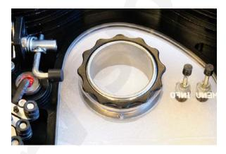
3. <u>Take off the adapter ring</u>: You will see a serrated ring. It's adapter ring to fasten the viewfinder adapter. Please use tools like Anthis Ring Nut Tool or pliers to unfasten it. Probably put a cloth on it to avoid any damage on the housing back cap.
