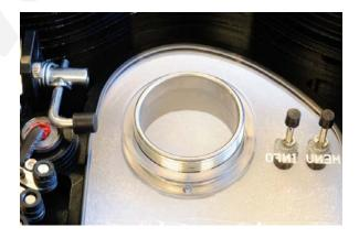
4. <u>Install Inon Viewfinder</u>: After taking off all Nauticam viewfinder and accessories, put Inon Viewfinder into it. Please check if it completely attached on the back cap of housings.
