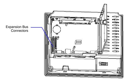
**Note:** To ensure compliance to CE Mark, the mounting screws must be used when installing an expansion card.
