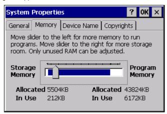
2. On the **Memory** tab, drag the slider to divide the DRAM into **Storage** and **Program** memory.
