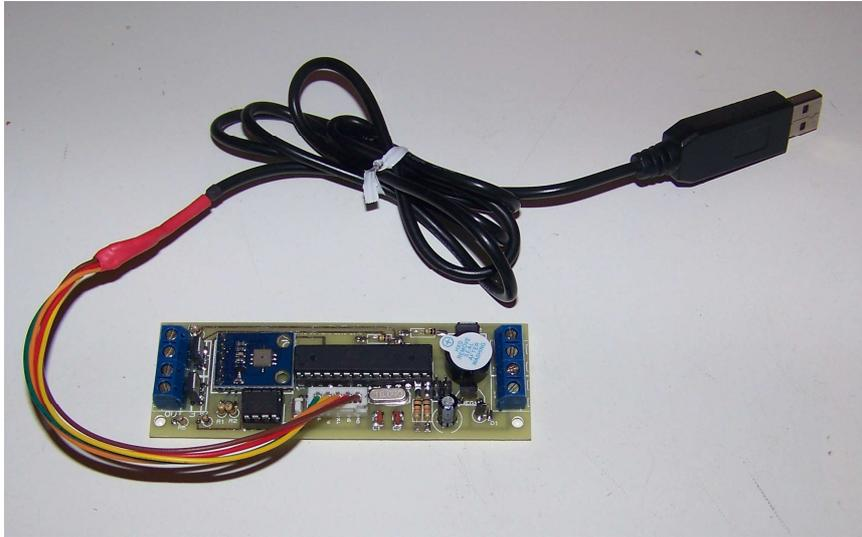
The altimeter should be beeping away doing its continuity test. A beeping altimeter does not mean an established communication.
