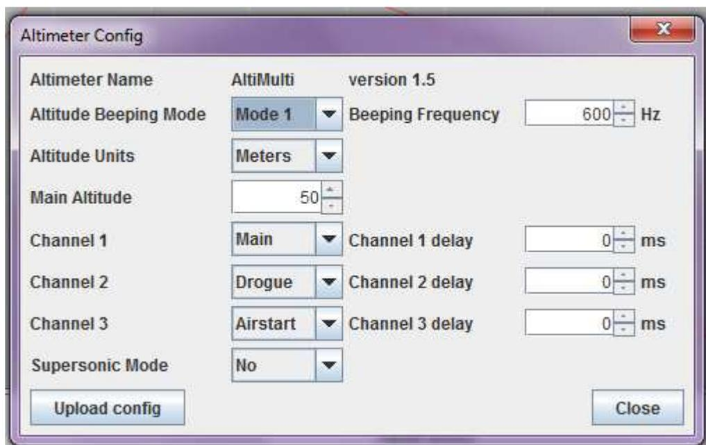
This retrieves for information the altimeter name and version (in the future it will be able to connect to different altimeter with some sort of plug-in mechanism).
