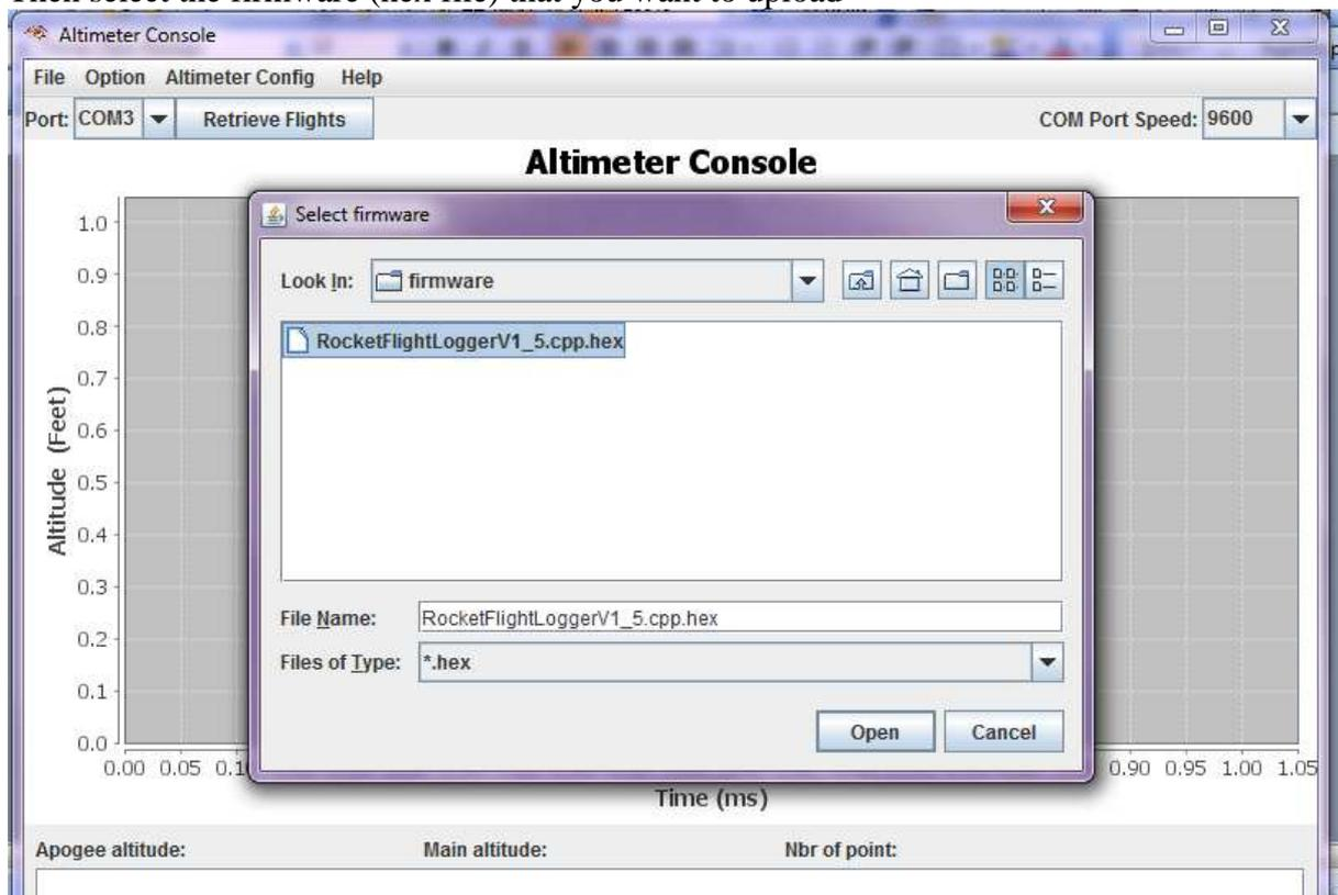
Press the altimeter reset button and click on open just after that. The program then upload, make sure you check the message window for errors or success.
