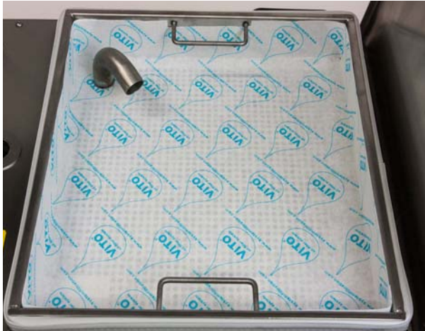
Don't leave gaps between the filter and the edges of the filter basket! Filter empty
