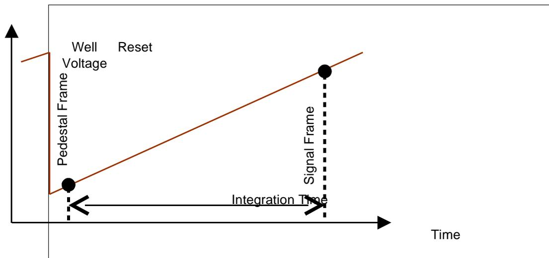
Figure 9 Illustration of Correlated Double Sampling's Pedestal and Signal Frames
