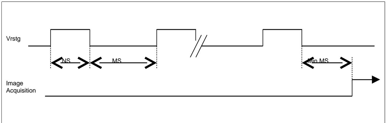
Figure 8 Background Reset Timing Diagram
