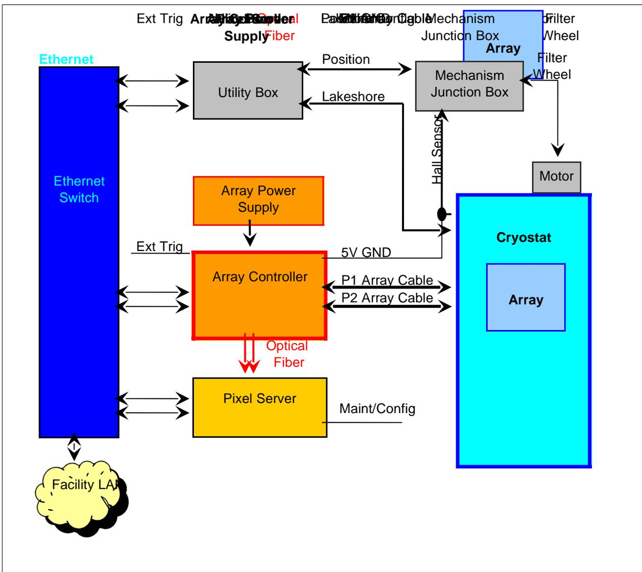
Figure 7 Block Diagram of Instrument Control Electronics
