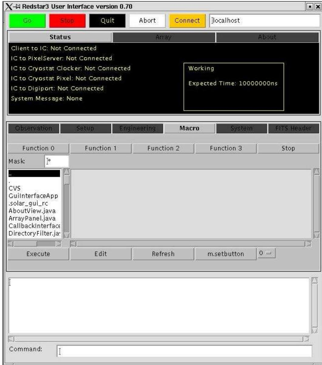
Figure 19 Screen Capture: Array Control GUI Macro Tab
