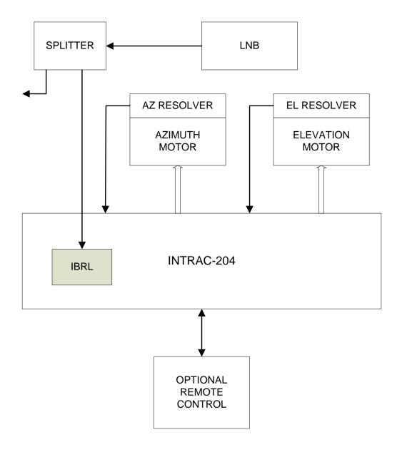
The Elevation & Azimuth resolvers provide antenna pointing information and the IBR-L beacon receiver provides tracking signal strength. (A signal strength derived dc voltage from an external receiver may be used in place of the IBR-L).
