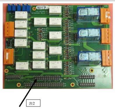
The ribbon cable is connected to the connector J12 identified by an arrow in the picture above. The ribbon cable has a connector at the end and one a few centimetres in from the end. If the 18v is not required then connect the ribbon to the card using the end connector. If 18v is required then connect the ribbon to the card using the other connector.
