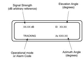
In normal operation mode (i.e., not in menu mode) the display shows the four factors as in the above diagram. In menu mode the options of the currently selected branch of the menu tree are displayed in one or two lines. **OPERATIONAL MENU**
