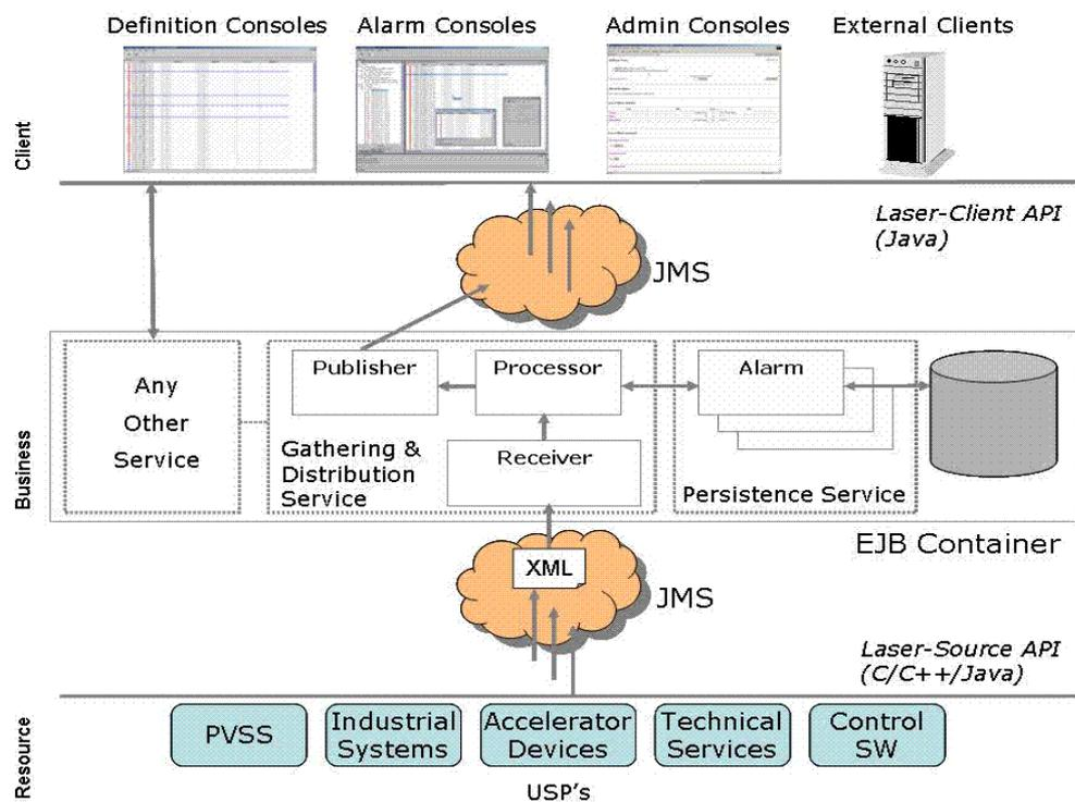
Figure 1: The architecture of the LASER alarm system
