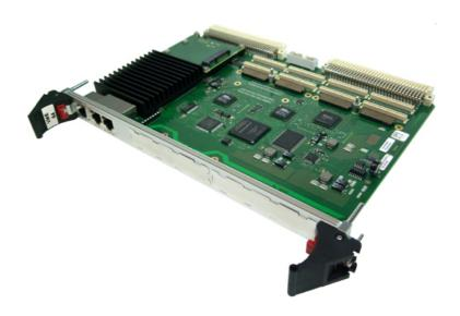
The A21C is a Freescale<sup>™</sup> QorlQ<sup>™</sup> based single-board computer for embedded industrial applications. The SBC features full VME64 support and can be used as a master or a slave in a VMEbus environment. The A21C provides 1 MB local dual-ported SRAM for slave access and communication between the local CPU and another VMEbus master.
