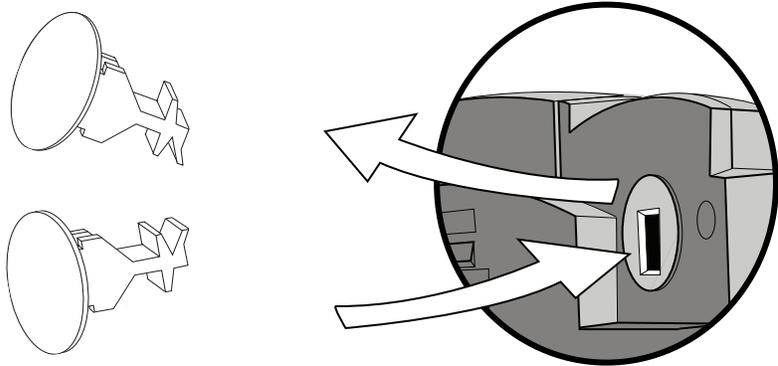
3. Using wall anchors (not included), fasten the base stand with the mounting tab facing up.
