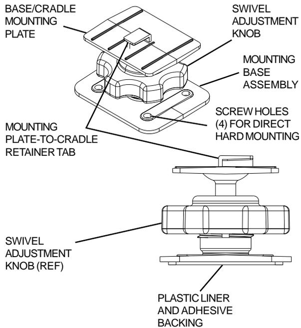
**NOTE:** Allow a 72-hour period for the adhesive backing to cure completely.
