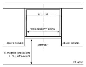
This type of hood must be installed inside a wall unit or similar support.
