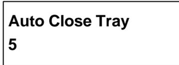
Here 5 means that it will take 5 seconds to close the writer's tray automatically after copying finishes and the tray is ejected. Besides 5 seconds, there are 10, 15, 20, 25, 30, 35, 40, 45, and 50 seconds for choice. If you have set one or all seven writers in function 11.4, and choose 10 seconds here, then one writer's tray or all seven writers' trays will be closed in 10 seconds after copying finishes.
