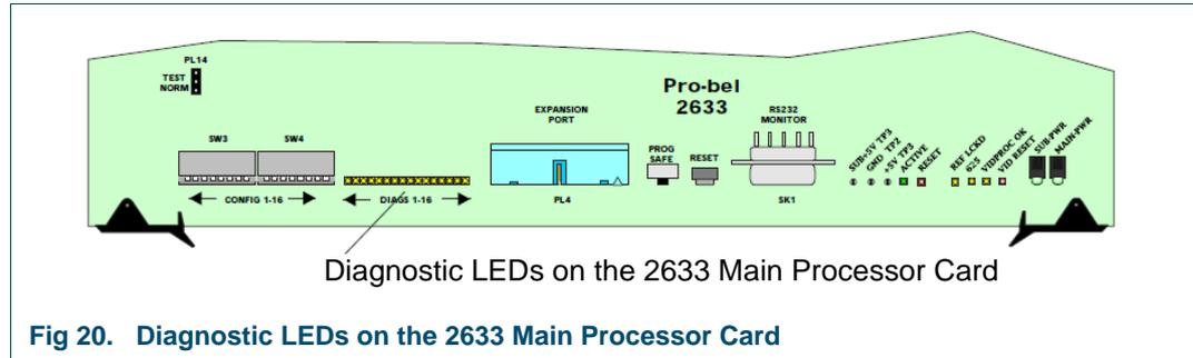
Fig 20. Diagnostic LEDs on the 2633 Main Processor Card
