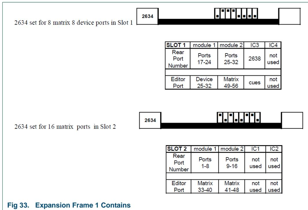
Fig 33. Expansion Frame 1 Contains
