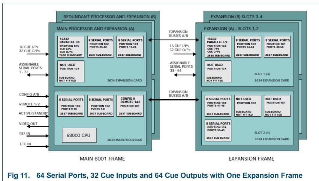
**Fig 11. 64 Serial Ports, 32 Cue Inputs and 64 Cue Outputs with One Expansion Frame**
