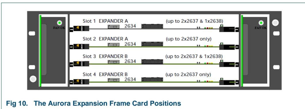
Fig 10. The Aurora Expansion Frame Card Positions
