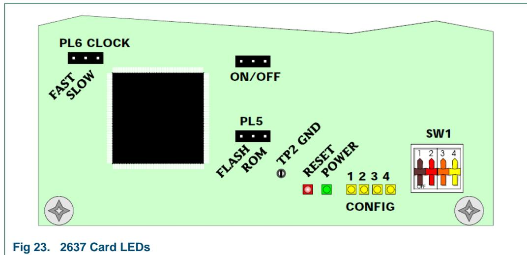
Fig 23. 2637 Card LEDs
