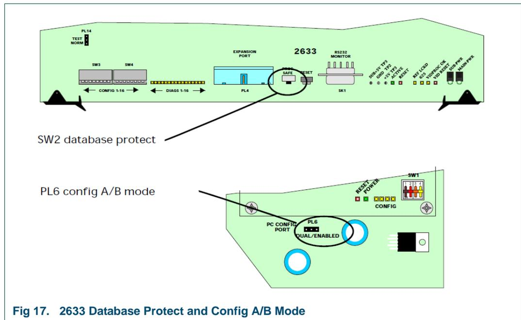
**Fig 17. 2633 Database Protect and Config A/B Mode**
