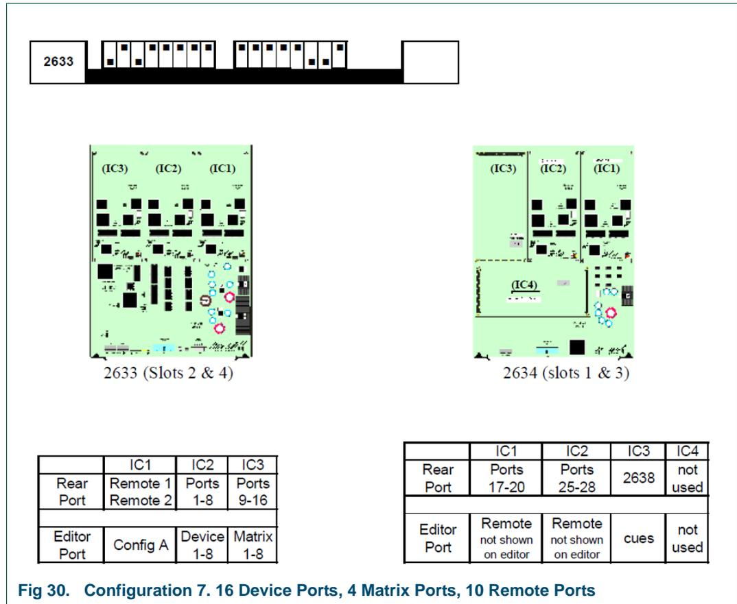
**Fig 30. Configuration 7. 16 Device Ports, 4 Matrix Ports, 10 Remote Ports**
