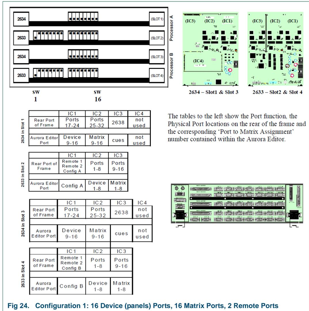
**Fig 24. Configuration 1: 16 Device (panels) Ports, 16 Matrix Ports, 2 Remote Ports**
