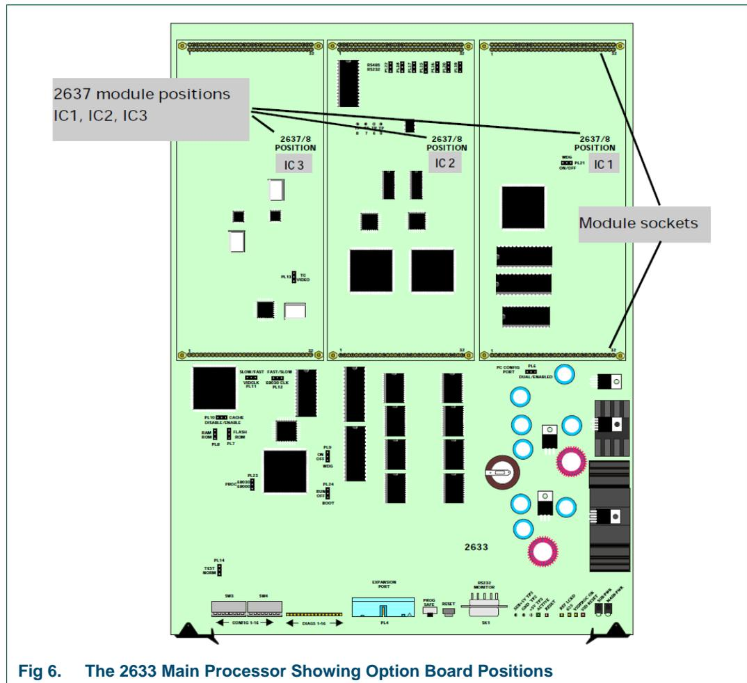
Fig 6. The 2633 Main Processor Showing Option Board Positions
