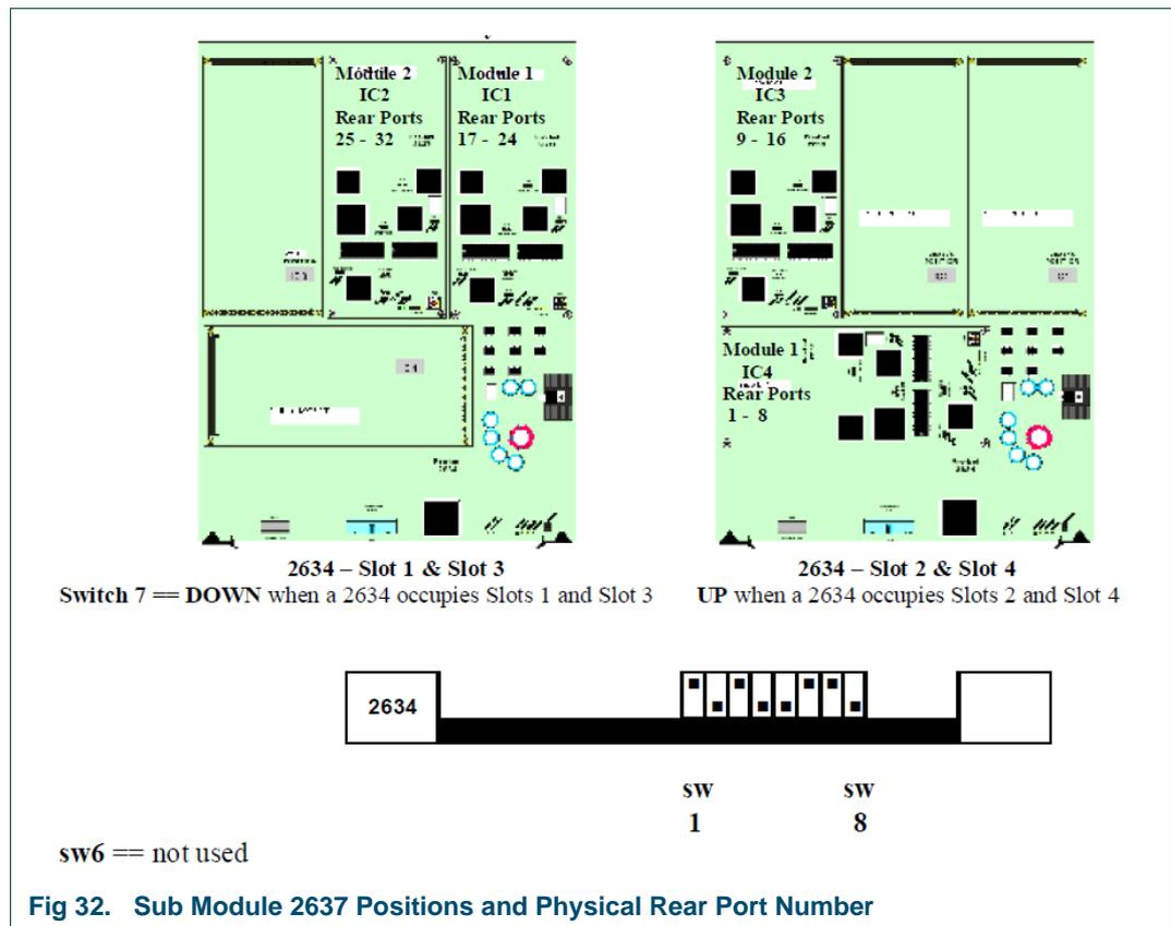
Fig 32. Sub Module 2637 Positions and Physical Rear Port Number
