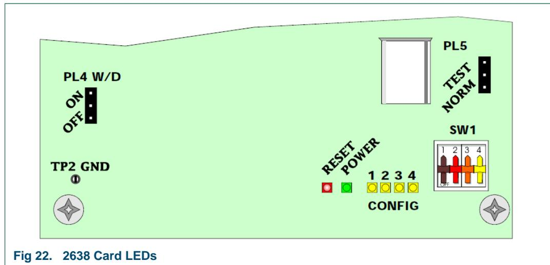
Fig 22. 2638 Card LEDs
