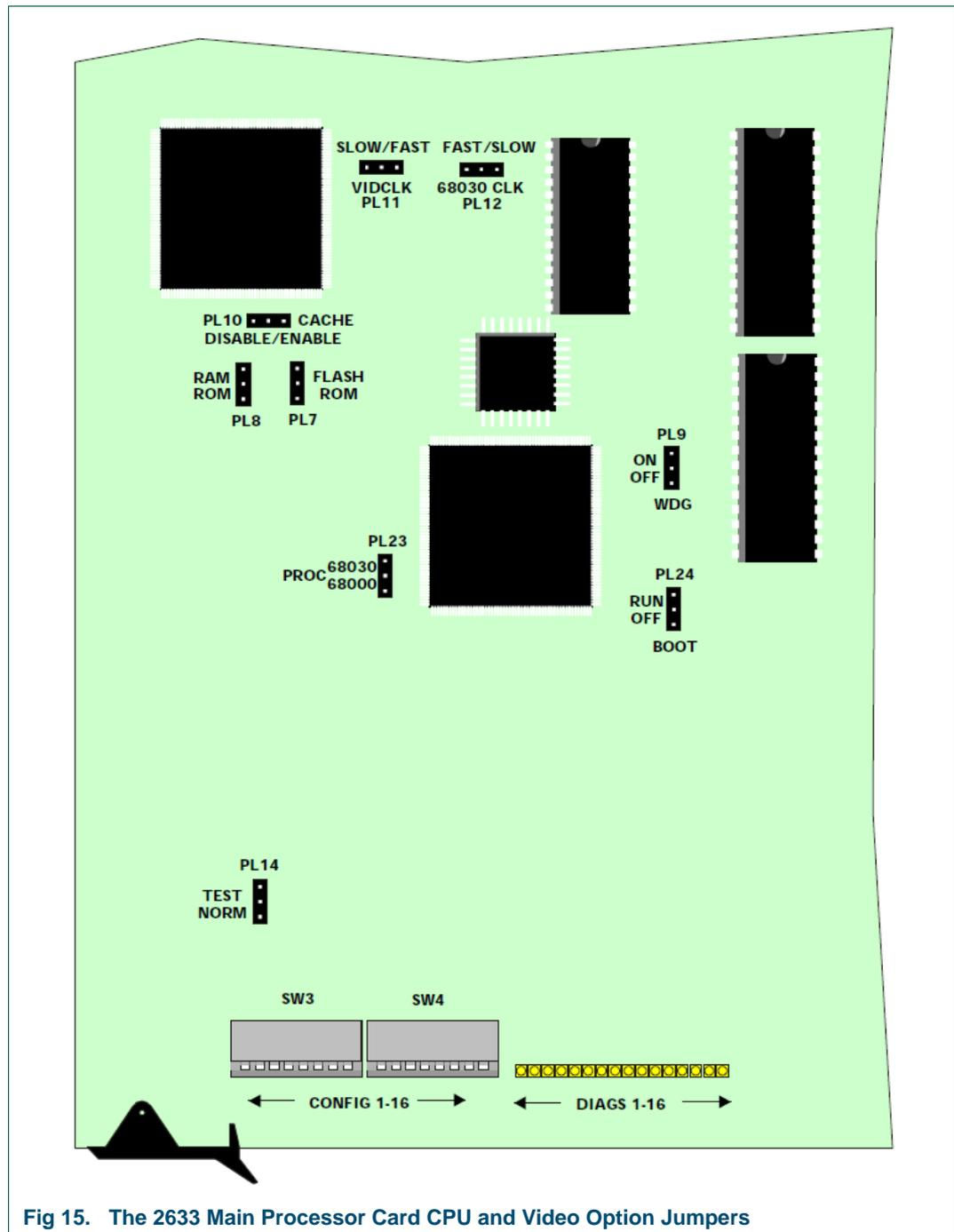
Fig 15. The 2633 Main Processor Card CPU and Video Option Jumpers
