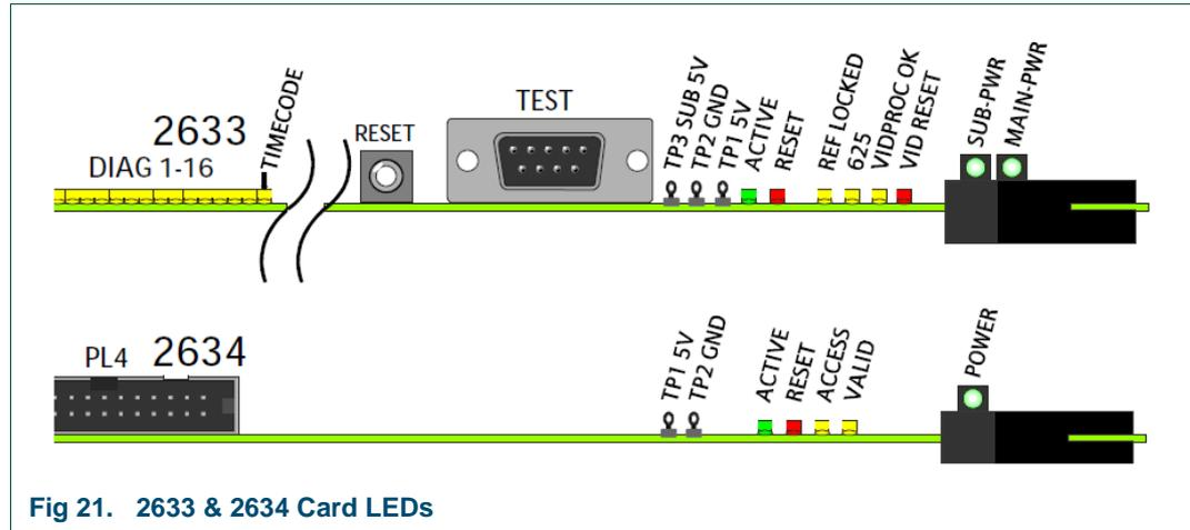
Fig 21. 2633 & 2634 Card LEDs
