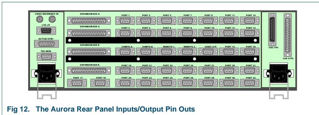
Fig 12. The Aurora Rear Panel Inputs/Output Pin Outs
