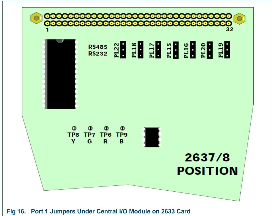
Fig 16. Port 1 Jumpers Under Central I/O Module on 2633 Card
