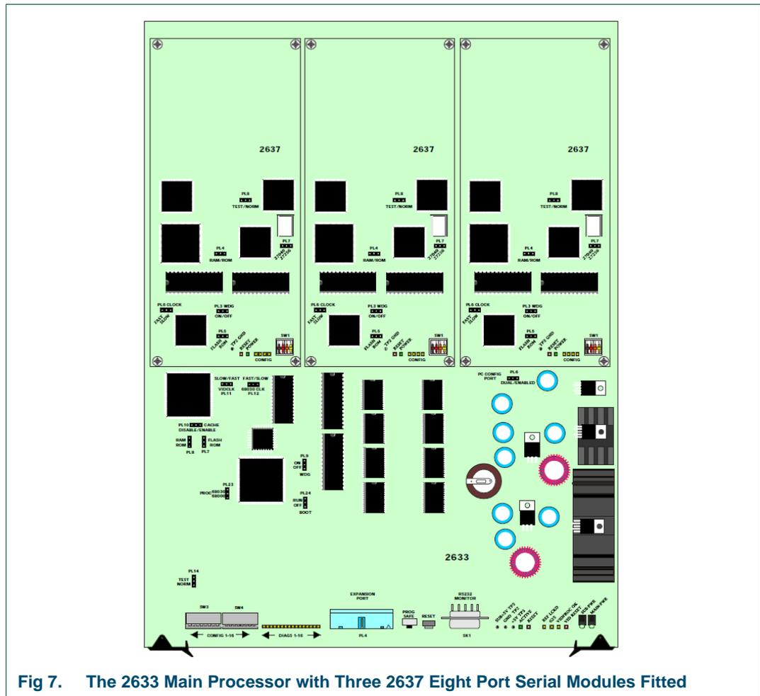
**Note:** Module orientation (DIP switch nearest board handles) when fitting modules. Each module should be a gentle push-fit into its connectors. Four screws retain each module in position.
