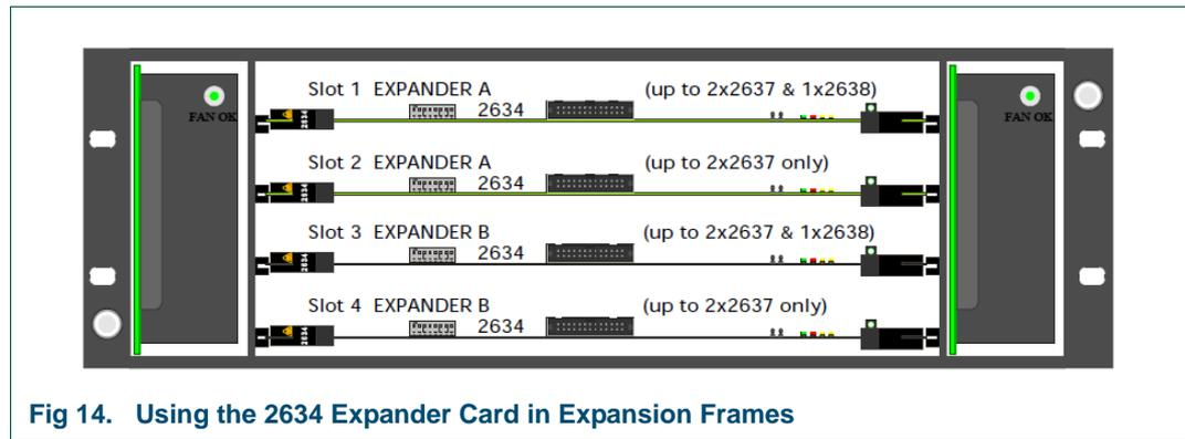
**Fig 14. Using the 2634 Expander Card in Expansion Frames**
