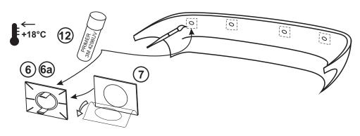
Remove the protective film from the adhesive (7) and apply it to the bracket (6 or 6a) or snap the bracket (8 or 9) in the hole from the outer part of the bumper.
