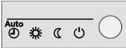
Press the button to select the different heating modes. The selected mode is indicated by a bar beneath the relative symbol.
