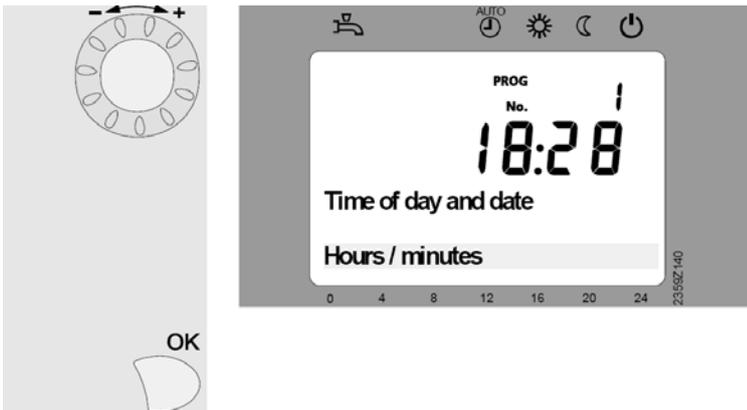
In the lower half of the display the first operating row of the 'Time and date' page is displayed. Rotate the knob until the 'Hours/minutes' operating row is displayed.
