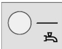
The button is used to enable and disable the heating of domestic tap water (ACS). The selected choice is indicated by a bar placed in conjunction with the relative symbol.
