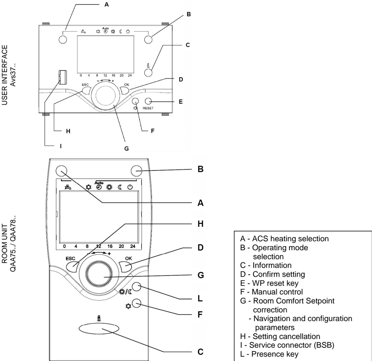
**Figure 2** Description of the AVS37... user interface controls and for room units QAA75.../QAA78...
