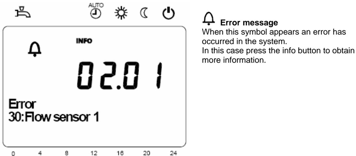
Figure 5 Viewing the error messages on the display
