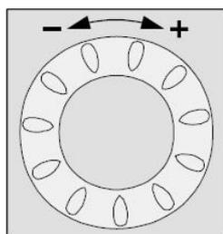
The heating setpoint, or the cooling setpoint, are inserted depending on the current operating mode (if the system is in “Heating” mode then the change will affect the heating setpoint, if the “cooling” mode is selected then it will affect the Conditioning setpoint).
