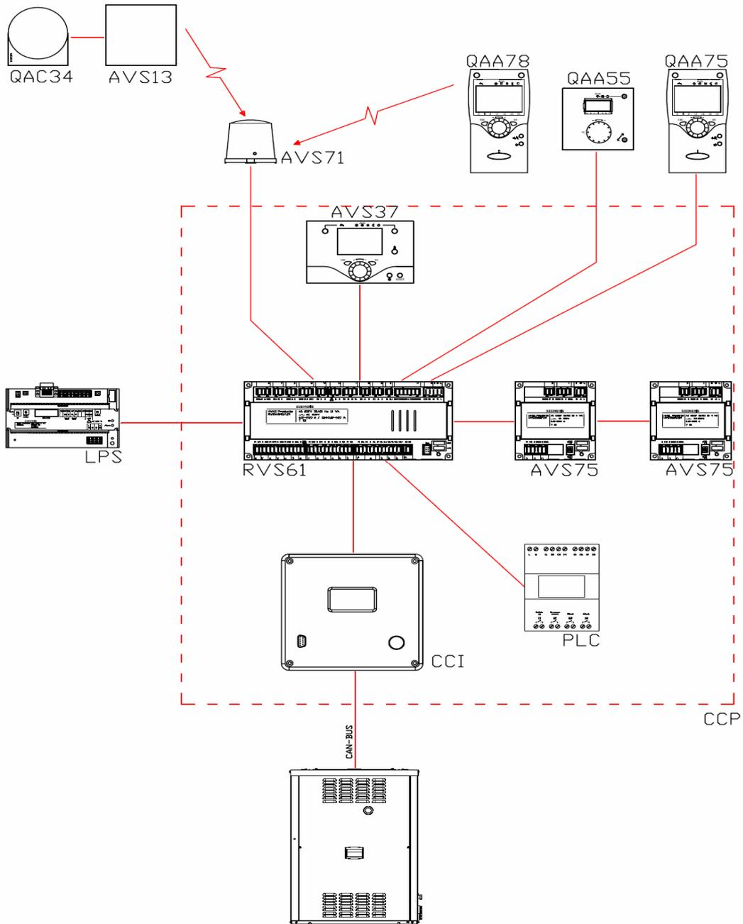
Figure 1 Initial description of the Comfort Control system
