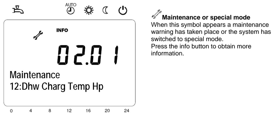
Figure 6 Viewing the error messages on the display
