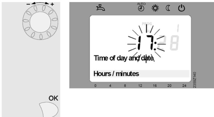
The hour display starts to flash. Rotate the knob to set the correct hour.
