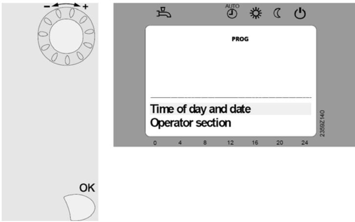
The lower part of the display shows a number of operating pages. Rotate the knob until the 'Time and date' operating page is displayed.
