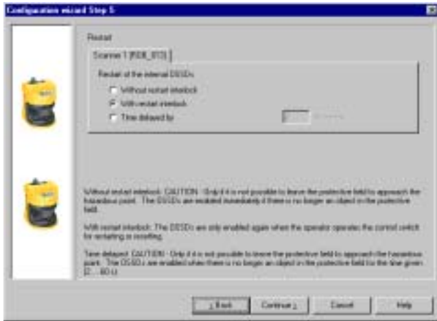
Figure 15: Dialog box for the configuration wizard based on the example of the SafeZone multizone
