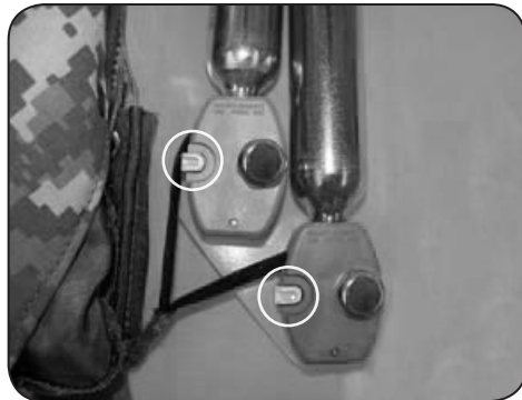
7.1.6 Installing the green safety clips.
