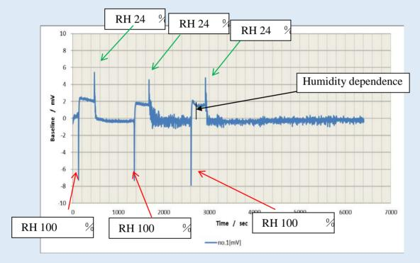
The transient spike response from the sensor for each humidity excursion was of approximately 5s in duration. The results here are expressed in mV from our recommended circuit, with 6mV being equivalent to 1 ppm Chlorine. The maximum amplitude of the spike when the humidity changed from low to high was 1.1 ppm equivalent, and -0.5ppm equivalent when humidity was changed from high to low.
