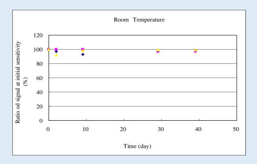
This data was generated in bench tests in a controlled clean environment. In service, in a real application, the long term stability will also be dependent on the environmental conditions of the application.
